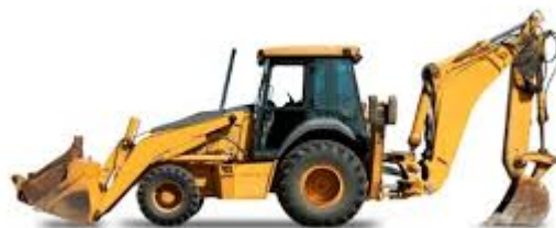
A Backhoe is used for light excavation work.
